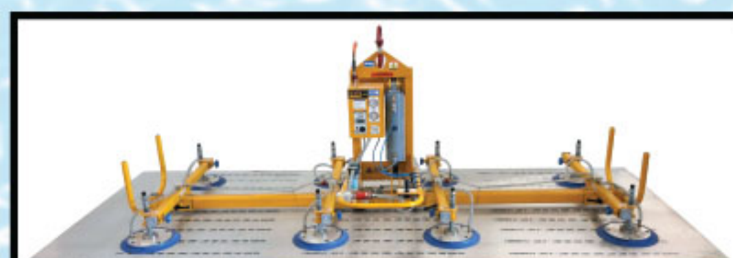
Vacuum Suction Lift Used For Aluminum/Stainless Steel (Scratch Free)
